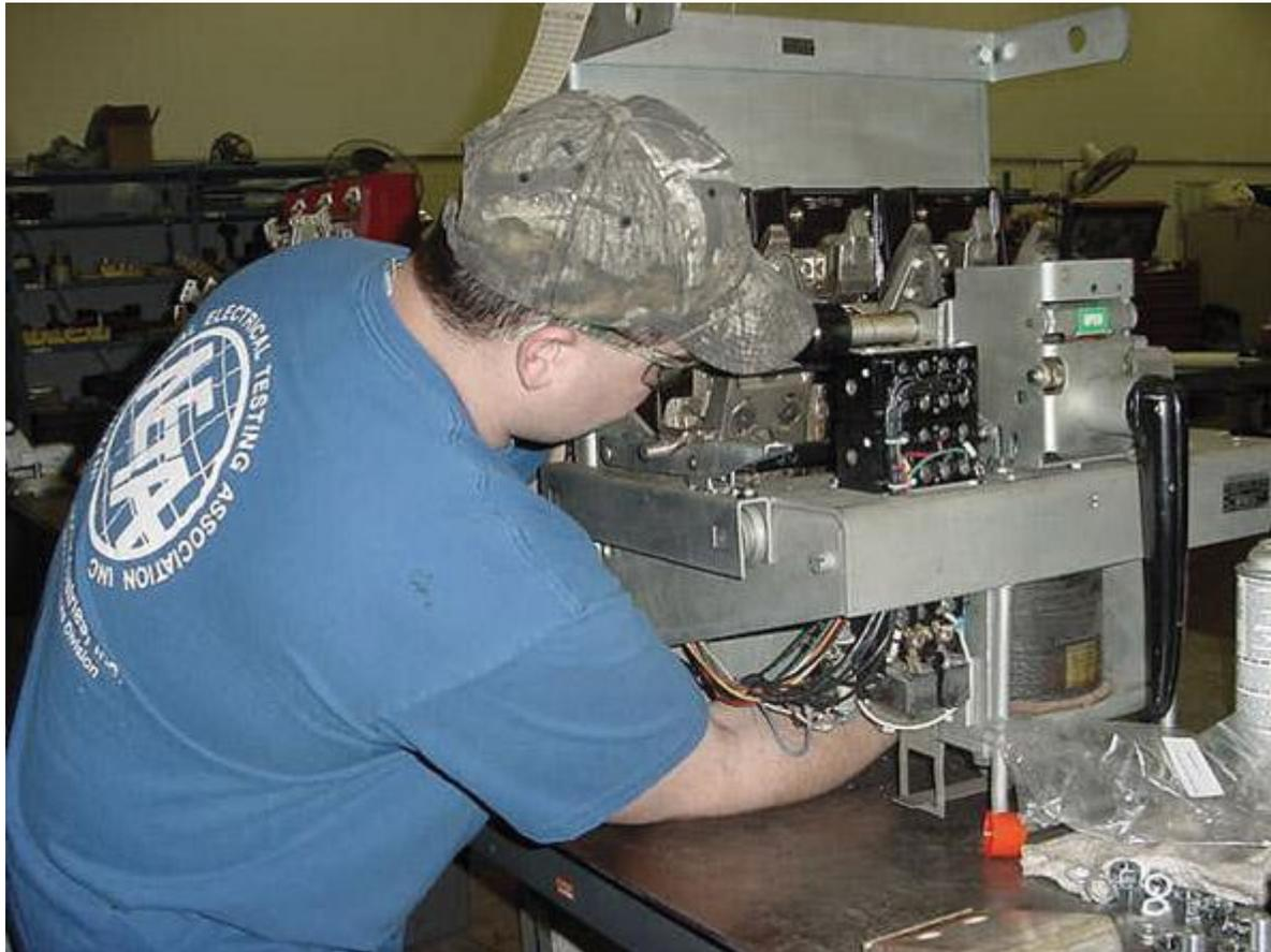
Photo 1. Will it trip, or won't it? Without the test or calibration decal, there's no way to tell when maintenance was last performed.
